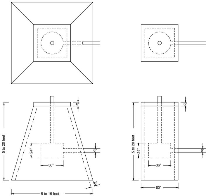
FIGURE 2. Possible pier designs, assuming a concrete structure.
