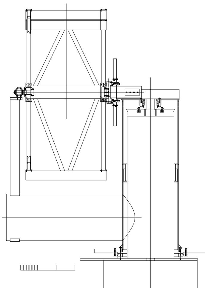
**FIGURE 1.** Telescope layout. The scale in the lower left represents a length of three feet.
