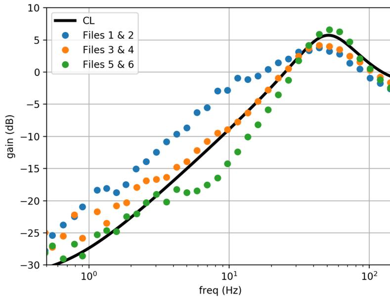
The significant difference between files 1&2 and 3&4 is striking because the configuration is the same. Files 5&6 use a larger gain and a damping parameter, which is not modelled here.
