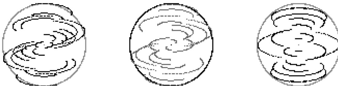
**FIGURE 3.**  $U - V$  coverage with optimum 5-telescope configurations. Left: restricted Mt. Wilson Y, Center: unrestricted Mt. Wilson Y. Right: unrestricted classical Y. The outer circle represents a 354 m separation, as in the original CHARA Y.
