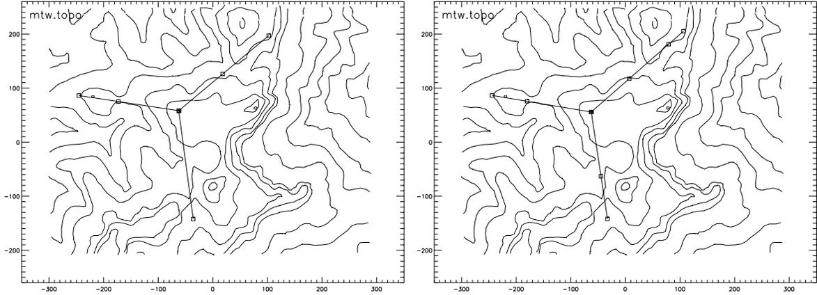
**FIGURE 2.** Mount Wilson site with optimum “restricted” 5- and 7-telescope configurations.
