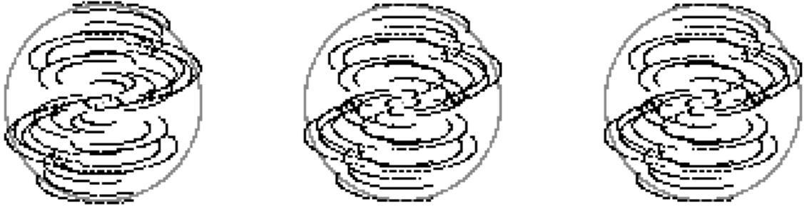
**FIGURE 4.**  $U - V$  coverage with optimum 7-telescope configurations. Left: restricted Mt. Wilson Y, Center: unrestricted Mt. Wilson Y. Right: unrestricted classical Y.
