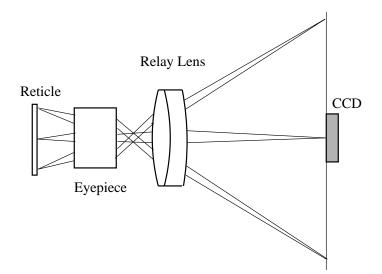
FIGURE 1. Reimaging the telescope image and the reticle onto a CCD by a relay lens.
