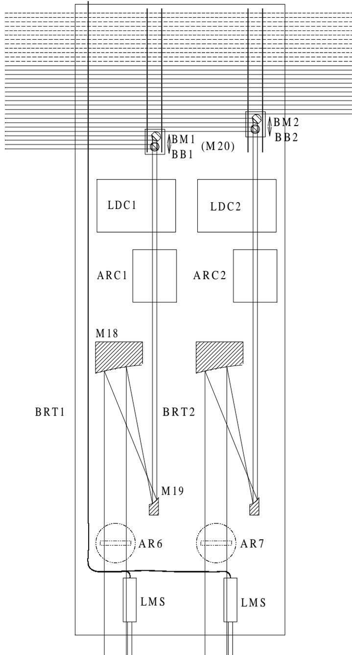
**FIGURE 4.** Schematic of the one of the beam sampling tables in the OPLE area. The metrology systems while shown here, are part of the OPLE cart contract with JPL.
