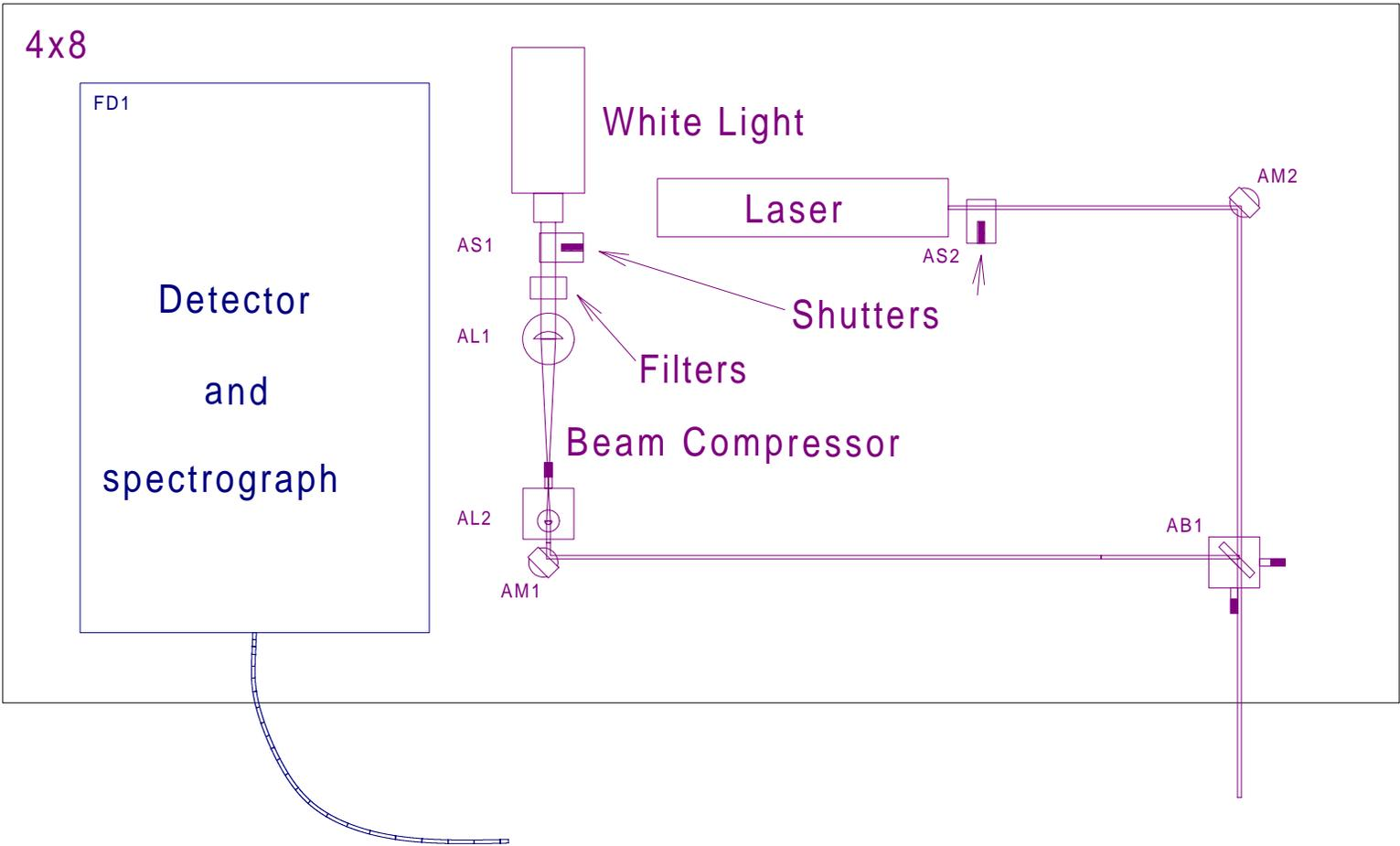
**FIGURE 1.** Schematic of the alignment optics table in the BCL.
