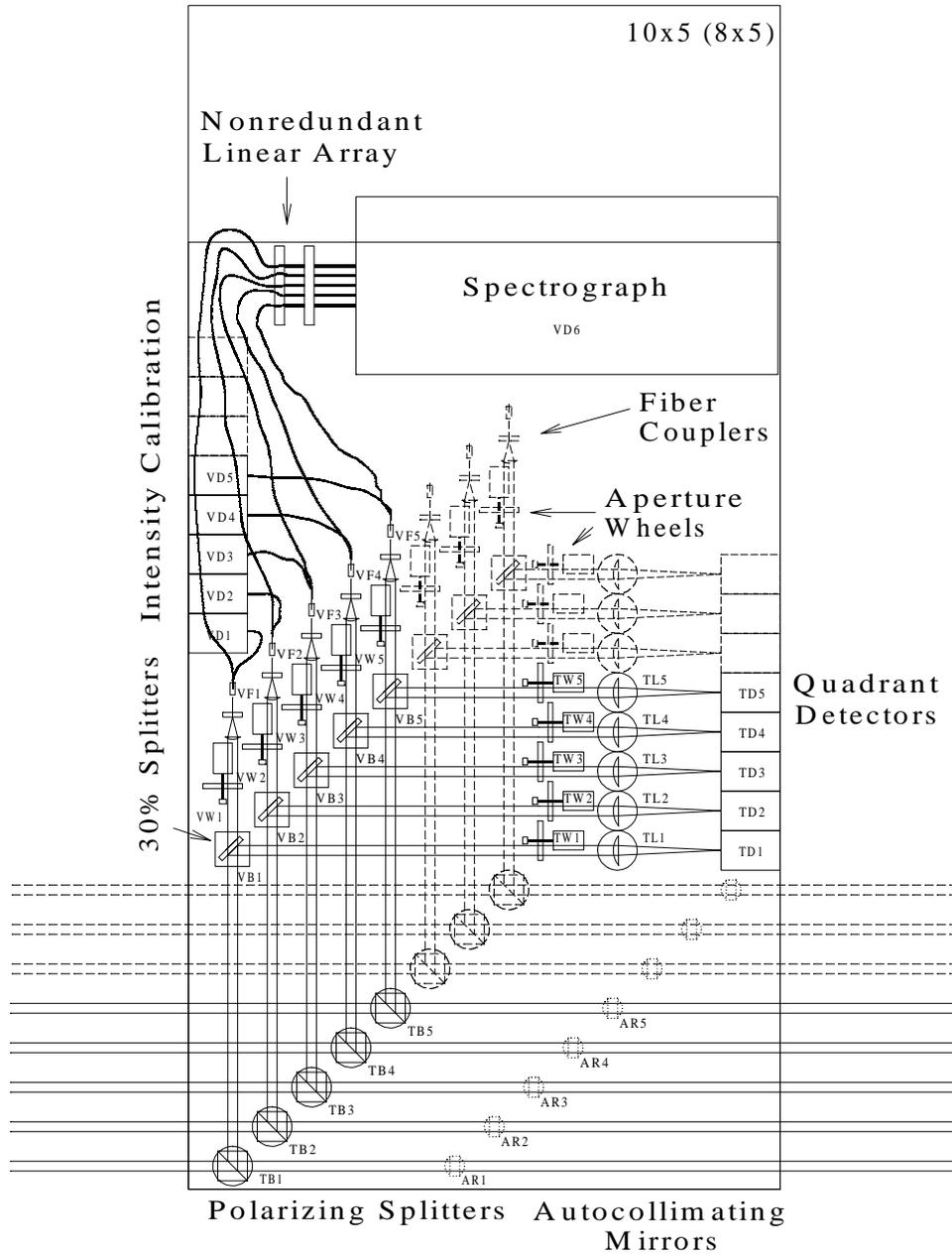
**FIGURE 3.** Schematic of the Tip/Tilt detector and imaging table in the BCL.
