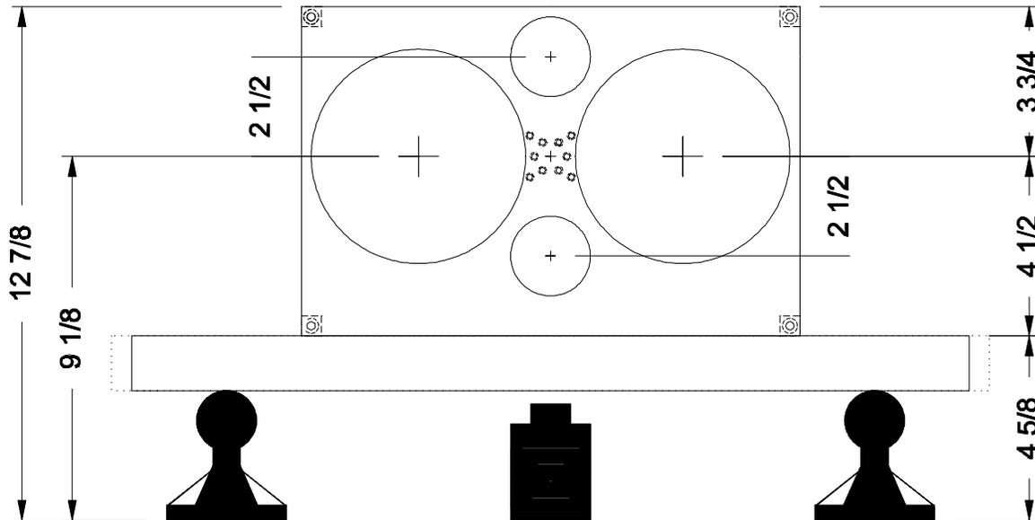
FIGURE 2. Nominal dimensions for the OPLE cart face plate.
