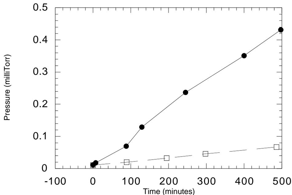
**FIGURE 1.** Vacuum test of two candidate tube bands. The upper curve (more rapid increase in pressure) corresponds to the NoHub commercial connector. The lower curve corresponds to the neoprene band, modeled after the NPOI concept.
