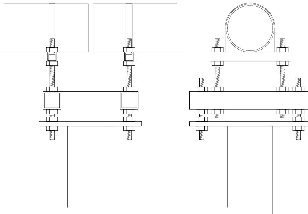
**FIGURE 2.** Support structure for the beam tubes. On top of a steel pole (diameter depends on height) a flat plate supports on threaded rod a 3 inch steel tube, which in turn supports a 1.5 inch section of U-channel. The channel anchors steel bands which hold the tube against the channel. This structure was designed for CHARA by Sea West Enterprises and Patrell Engineering Group.
