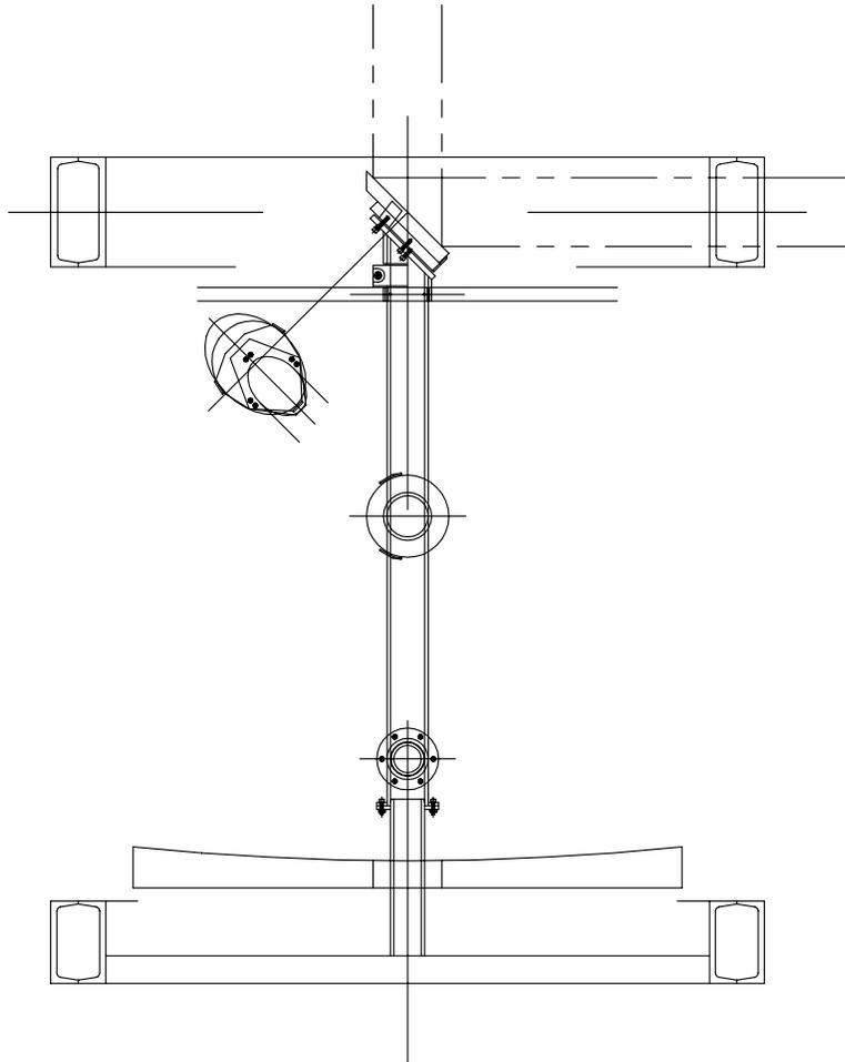
**FIGURE 4.** The tertiary mirror assembly.
