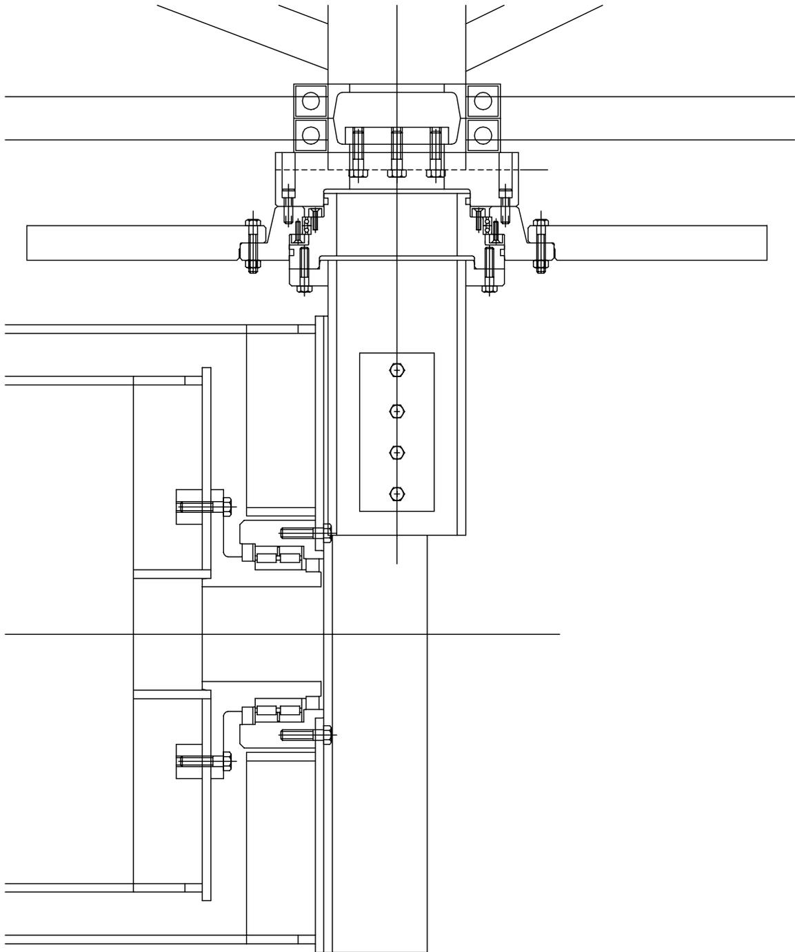
FIGURE 5. Azimuth and elevation bearings.
