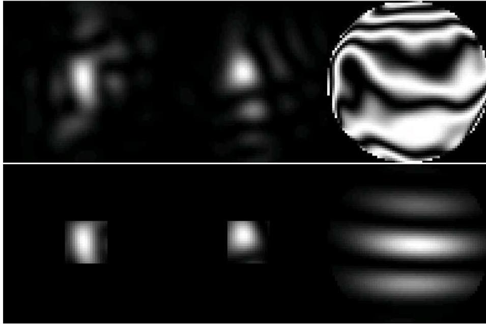
**FIGURE 1.** Two example frames from the simulation, both for  $r_0 = 3\text{cm}$ . The top plot shows the two image planes and the resulting fringe pattern without a spatial filter, and the bottom plot shows the same frame with a spatial filter of size  $2\lambda/D$ . In both cases a differential tilt has been imposed on the fringe pattern for display purposes only.
