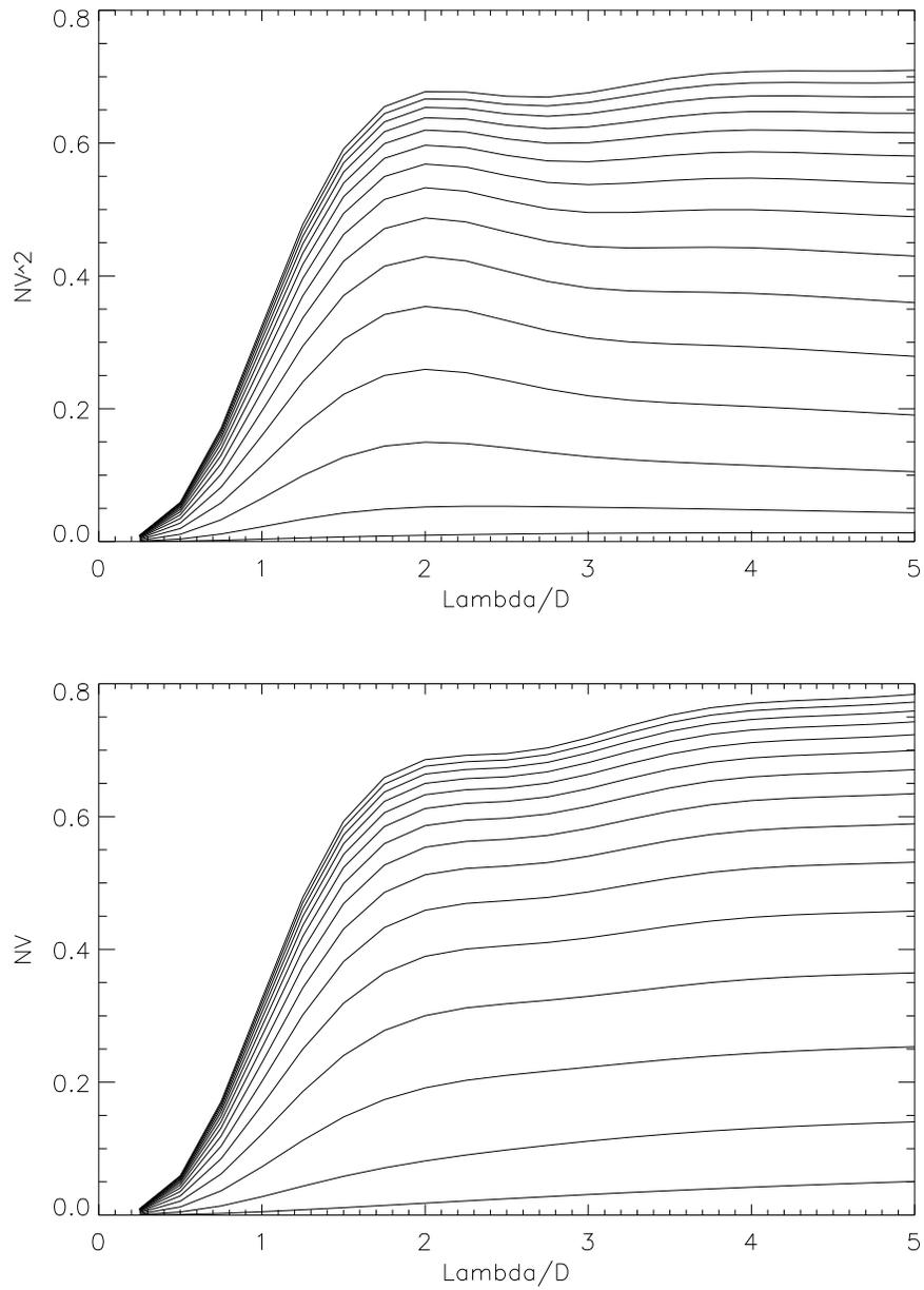
**FIGURE 4.** Final signal to noise ratio for a range of  $r_0$  values from 1 to 15cm. The top plot shows  $NV^2$ , while the bottom plot shows  $NV$
