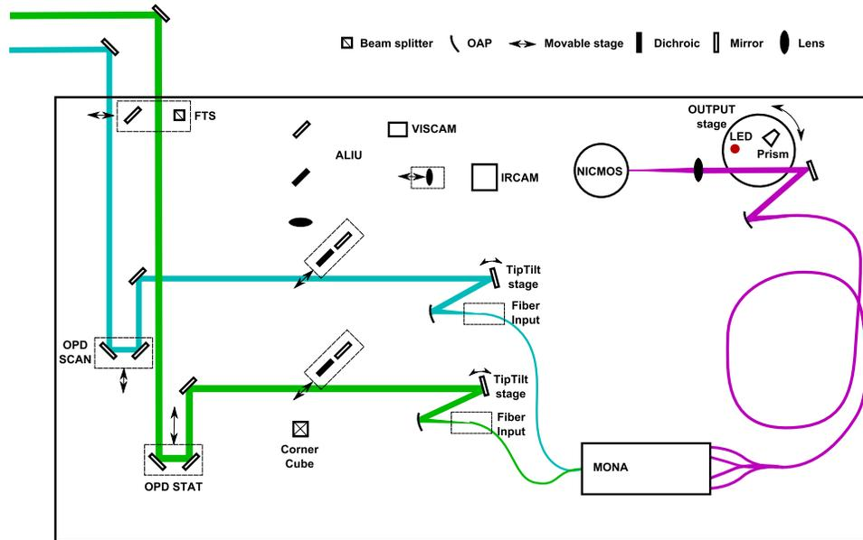
Fig. 2. JouFLU in the configuration used when observing. The alignment stages are out of the path of the beam and the OUTPUT stage is moved to the open position. Also shown for completeness are the optics of the alignment portion of the bench, see Fig. 7 for their use. The Fourier Transform Spectrograph beamsplitter is removed, see Fig. 5.
