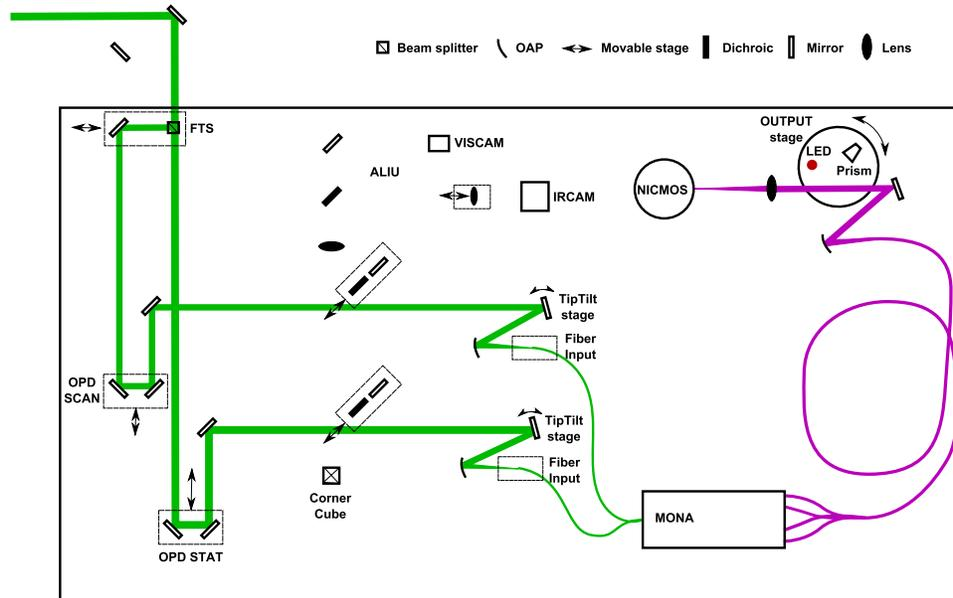
Fig. 5. FLUOR in the configuration used when calibrating with the Fourier Transform Spectrograph (FTS). The alignment stages are moved out, the FTS beamsplitter is moved into place, and OPD STAT changes position to compensate for the change in OPD.
