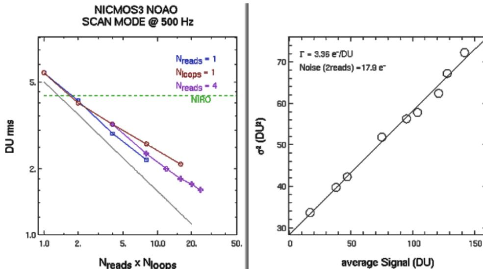
Fig. 11. Early tests of the NICMOS camera showing effect of changing the number of times a pixel is read/looped (Left) and the gain and readout noise under increasing amounts of flux (Right). Figures from Antoine Mérand, March 2007.
