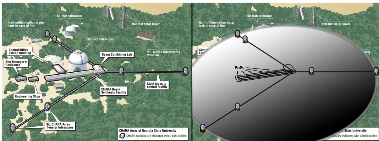
Fig. 1. Layout of the CHARA Array’s six telescopes, light pipes, and Beam Combining Lab within the context of the other facilities on Mt. Wilson (*left*). The illustration on the right shows the size of a mirror of equivalent resolving power to the CHARA Array. Also visible within the outline of the Beam Combining Lab are the “Pipes of Pan” (PoPs). Mirrors inserted at these points allow for various fixed intervals of large delay.
