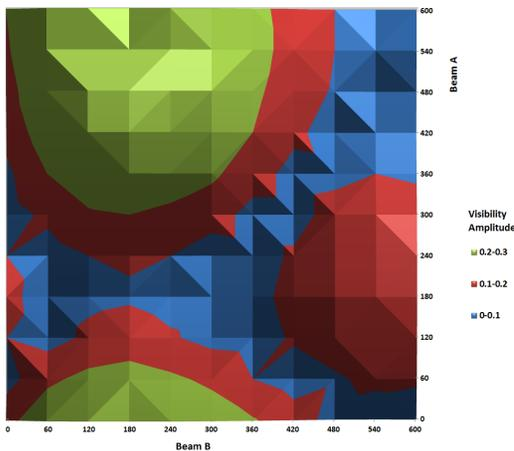
Fig. 6. The effects of adjustment of the fiber polarization for each of the two beams on white light fringe visibility. Each fiber has a knob which affects the bend of the fiber. Each knob was incrementally adjusted in steps of 60 arbitrary units to give 100 data points. Based on these results MONA was set to 480 and 180 for the top and bottom knobs, respectively.
