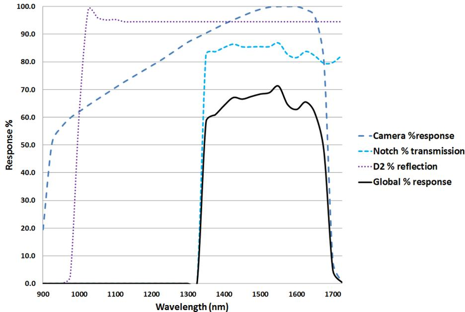
Fig. 9. The global response function for the H-band pupil imaging camera. Also plotted are the response functions for a single notch filter, the camera response function, and the dichroic (D2) reflection function. The global function is the product of the camera’s response, the two notch filters, and the D2 reflection.
