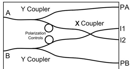
Fig. 3. The MONA fiber beam combiner consists of two Y-fiber couplers and one X-fiber coupler outputting one photometric channel for each beam and two interferometric channels total. Fiber polarization can be adjusted by changing the amount of bend to the fiber in the two loops.
