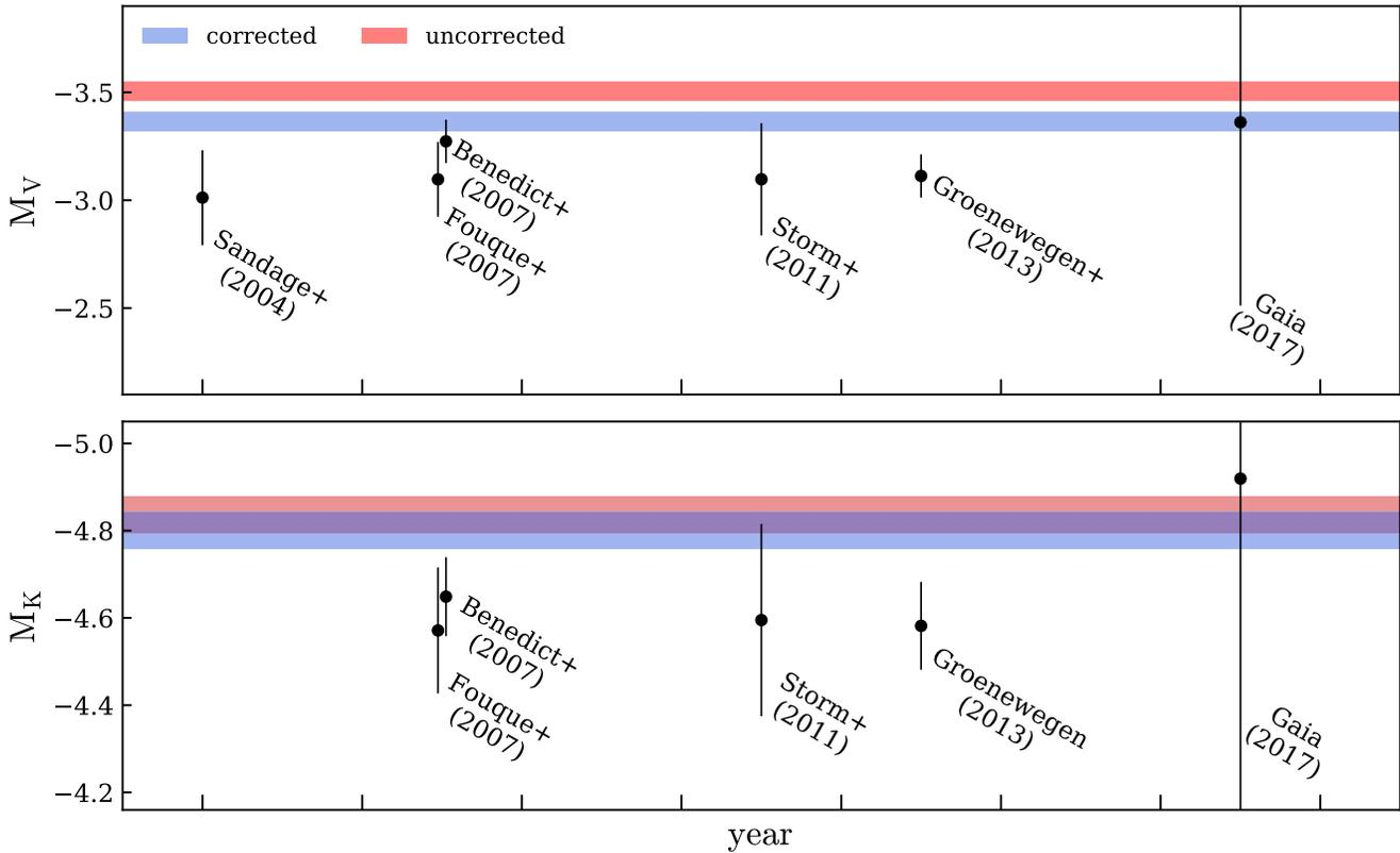
**Figure 3.** Comparison between the absolute magnitudes of V1334 Cyg predicted from literature P–L relations (black dots) and the present distance measurement (red and blue areas) in two photometric bands. The blue and red areas represent the measured absolute magnitude with and without the subtraction of the companion’s flux contamination, respectively. In the *K* band, these two regions overlap as the contribution of the companion is smaller.
