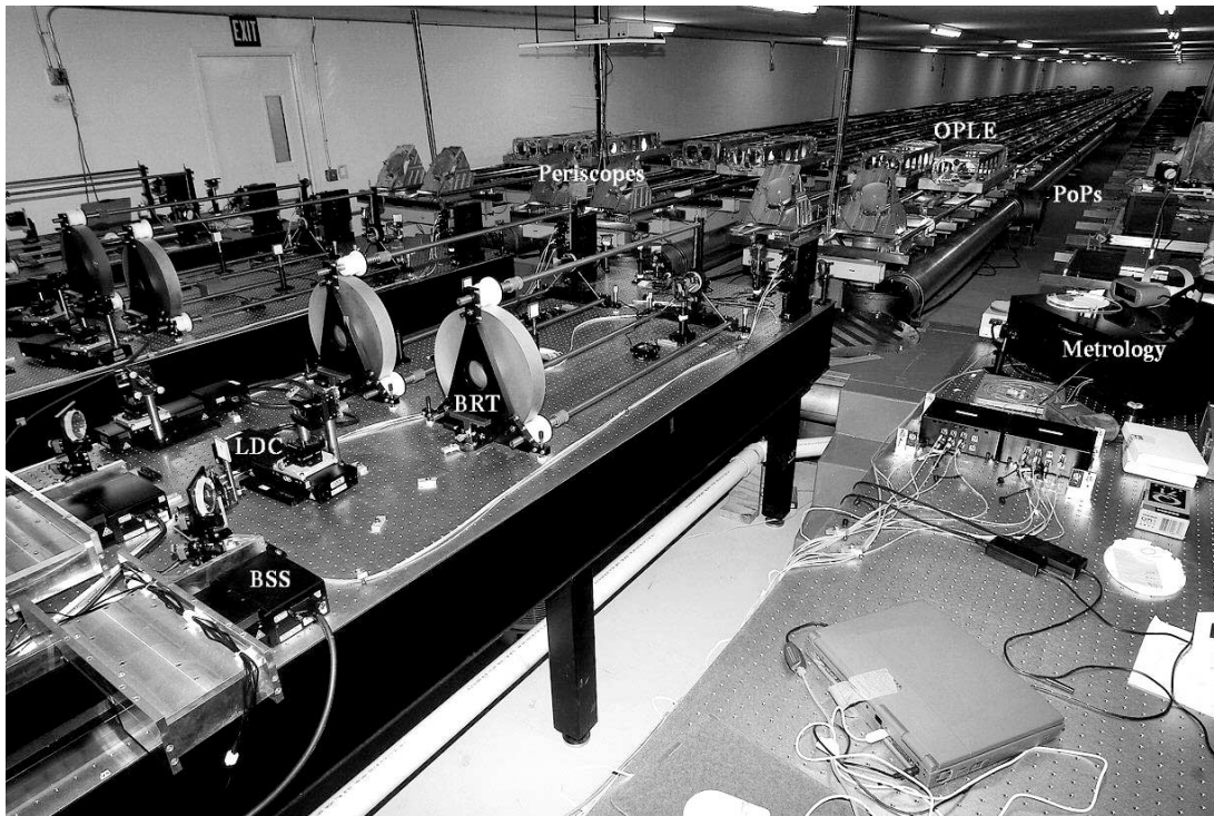
Fig. 7.—Delay line and beam management area. The PoPs, periscopes, OPLEs, BRTs, LDCs, and BSS system are clearly visible. Photograph by Steve Golden.
