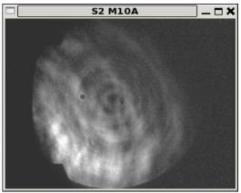
M10 alignment after re-centering the pupil. Note that it has shifted slightly from the nominal position. This is caused by some sort of pupil shift between the lab and the telescope, probably by the telescope dichroic being in back to front. The shift is smaller than many seen during the night.
