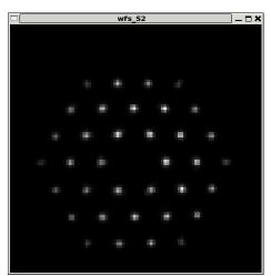
*TWFS spots after focusing the WFS/ACQ-parabola using the TWFS as a reference.*
