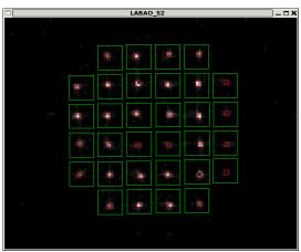
Blue LED beacon centered on LWFS. The focus of the beacon was set using the two-hole mask. Here it looks out of focus because we are using the old default flat.
