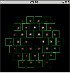
TWFS before adjusting WFS/ACQ parabola focus.
