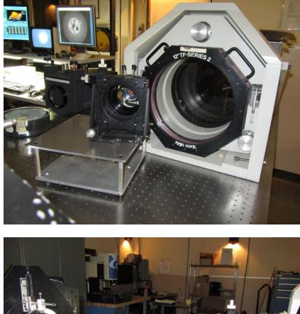
Figure 2. Photos of setup used. Photo at left, taken from parabola position, shows 12" TF with returning RS mounted just behind parabola focus. Lower photo shows parabola mounted with ½" wide polished ring mounted to it. Parabola was adjusted with ring perpendicular to outgoing beam before fine-tuning was performed to minimize aberrations.
