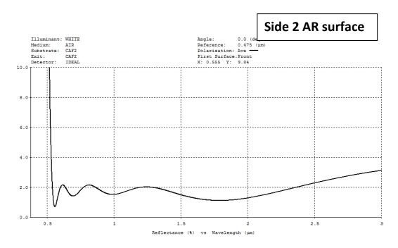
1. Calculated Ravg=1.7% for 0.55-2.45μm @ Odeg AOI
