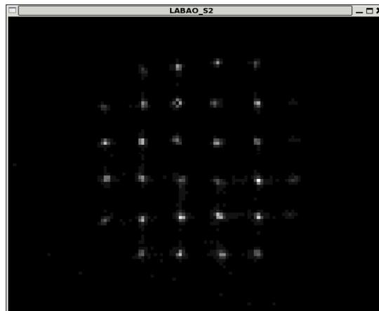
*Beacon centered on LWFS using M10 and Telescope dichroic. Spots on right are faint, we think, due to poor TWFS alignment.*
