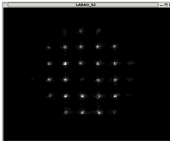
*Blue LED beacon on LWFS. The spots are well centered but one subaperture is faint because it is behind the central obscuration of the beacon. The pupil needs to move up and to the right.*
