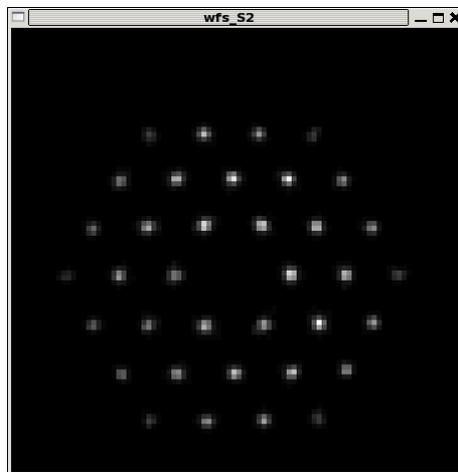
*TWFS spots after focusing the WFS/ACQ-parabola using the TWFS as a reference.*
