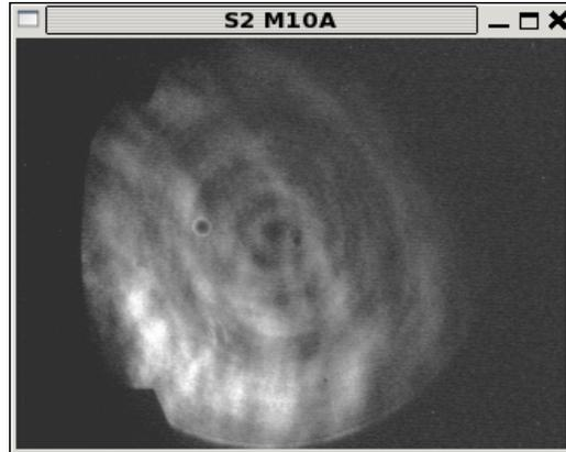
*M10 alignment after re-centering the pupil. Note that it has shifted slightly from the nominal position. This is caused by some sort of pupil shift between the lab and the telescope, probably by the telescope dichroic being in back to front. The shift is smaller than many seen during the night.*
