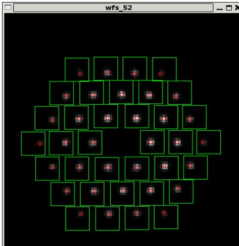
*TWFS before adjusting WFS/ACQ parabola focus.*
