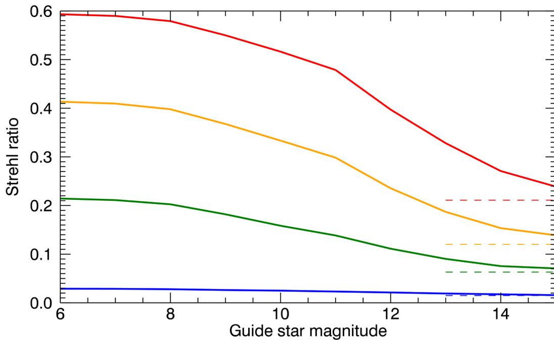
Figure 6: Strehl versus guide star R-magnitude for an open-loop tip-tilt system with an  $r_0$  at 550 nm of 0.10 m. The four colors represent R (blue), J (green), H (orange) and K (red) and the dashed lines show the performance with no correction.
