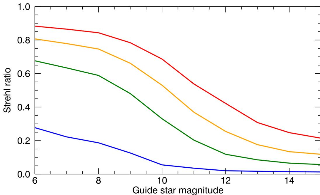
Figure 12: Strehl versus guide star R-magnitude for an open-loop 7x7 actuator DM system with an  $r_0$  at 550 nm of 0.10 m. The four colors represent R (blue), J (green), H (orange) and K (red).
