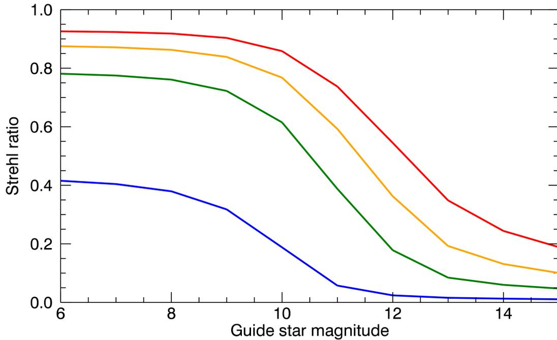
Figure 15: Strehl versus guide star R-magnitude for a closed-loop, 7x7 actuator DM system with an  $r_0$  at 550 nm of 0.10 m. The four colors represent R (blue), J (green), H (orange) and K (red).
