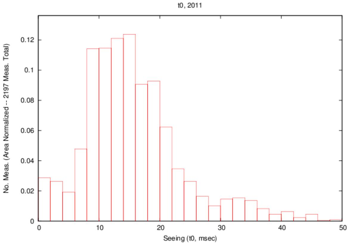
Figure 3: Measured  $\tau_0$  at 2300 nm.
