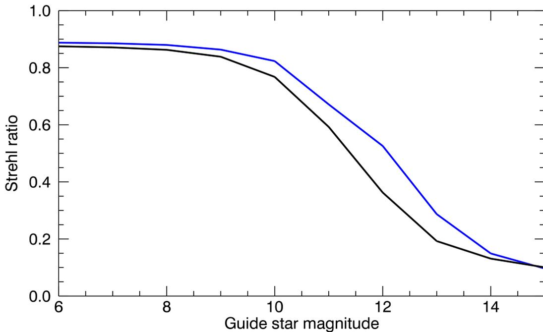
Figure 20: H-band Strehl versus guide star R-magnitude for a Shack-Hartmann wavefront sensor (black) and a pyramid sensor (blue). The value of  $r_0$  at 550 nm is 0.10 m.
