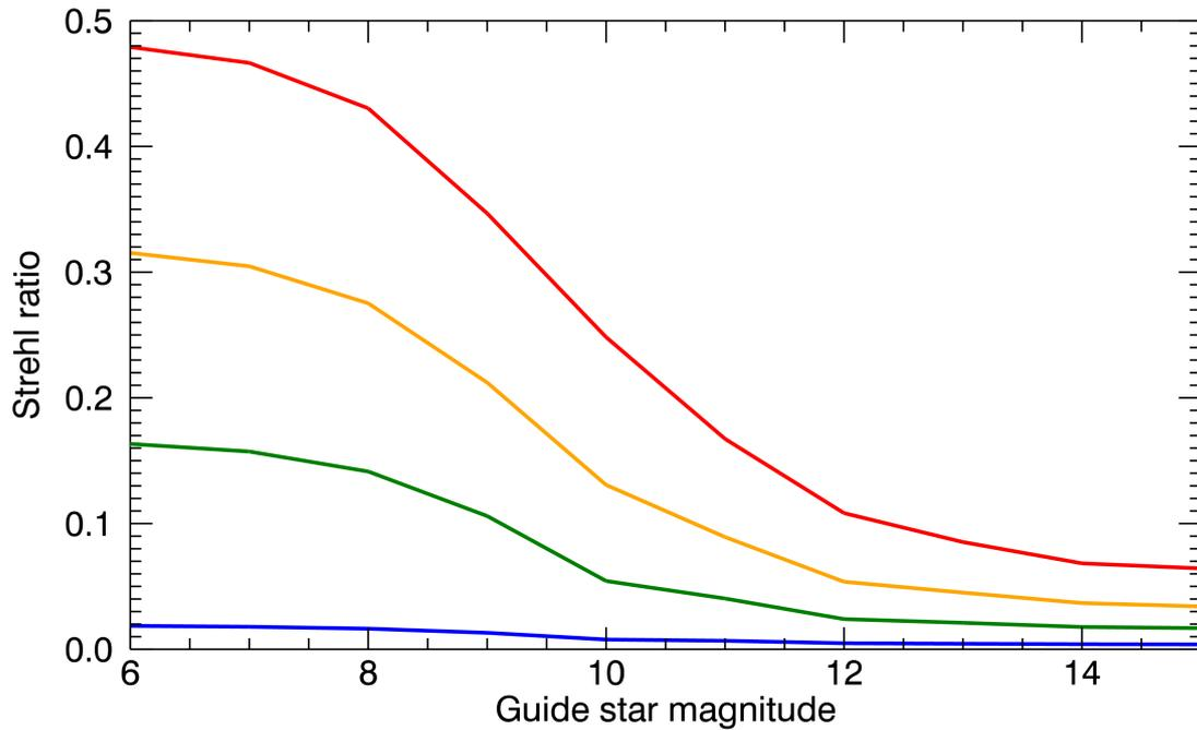
Figure 11: Strehl versus guide star R-magnitude for an open-loop 7x7 actuator DM system with an  $r_0$  at 550 nm of 0.05 m. The four colors represent R (blue), J (green), H (orange) and K (red).
