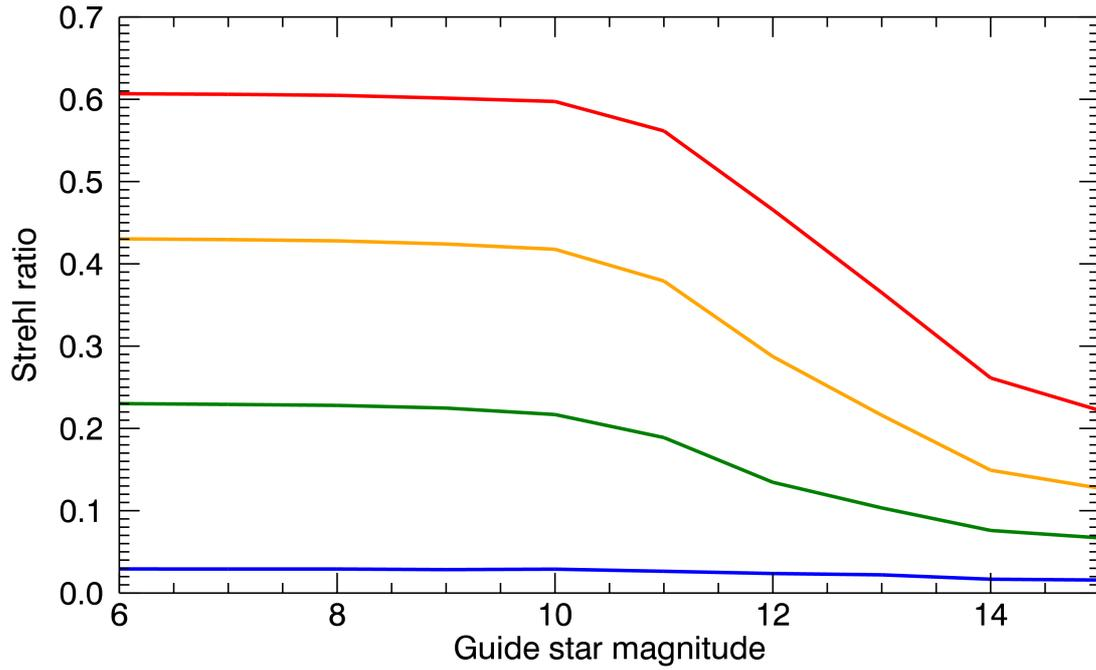
Figure 9: Strehl versus guide star R-magnitude for a closed-loop tip-tilt system with an  $r_0$  at 550 nm of 0.10 m. The four colors represent R (blue), J (green), H (orange) and K (red)..
