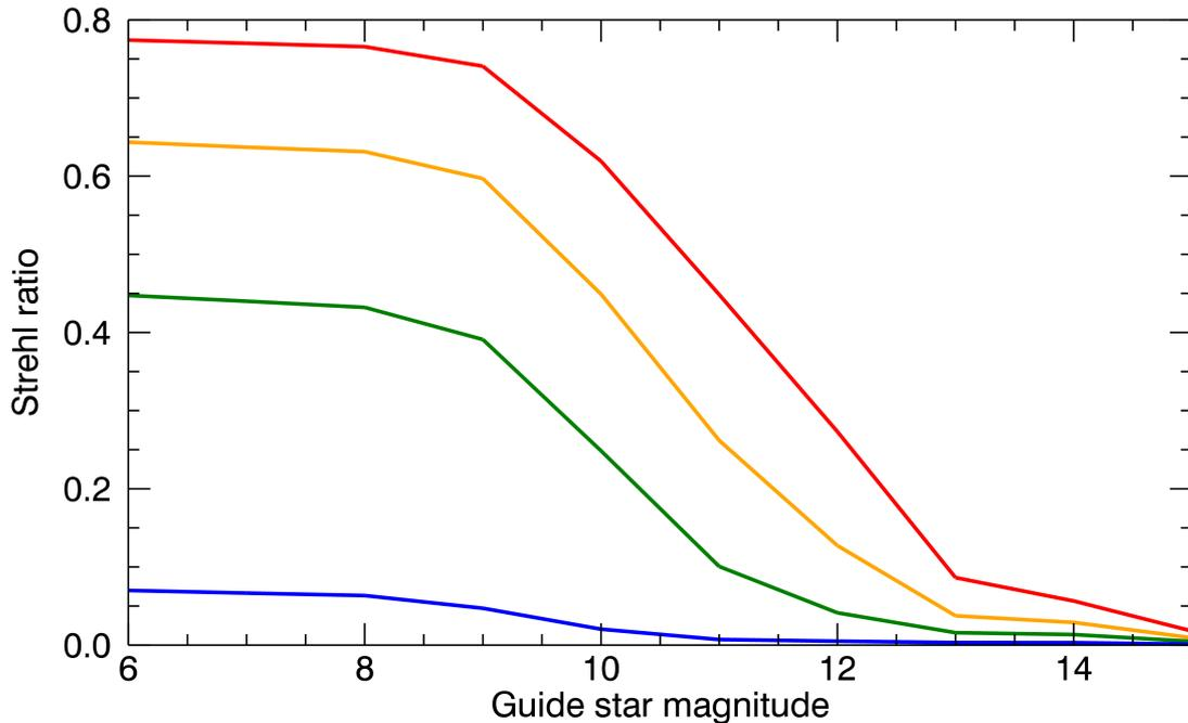
Figure 17: Strehl versus guide star R-magnitude for a closed-loop 7x7 actuator DM system with an  $r_0$  at 550 nm of 0.05 m. The four colors represent R (blue), J (green), H (orange) and K (red).
