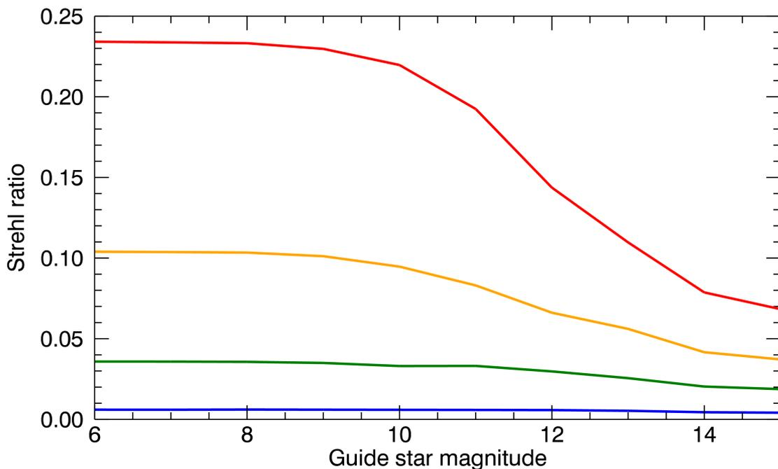
Figure 8: Strehl versus guide star R-magnitude for a closed-loop tip-tilt system with an  $r_0$  at 550 nm of 0.05 m. The four colors represent R (blue), J (green), H (orange) and K (red).
