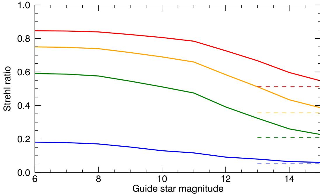
Figure 7: Strehl versus guide star R-magnitude for an open-loop tip-tilt system with an  $r_0$  at 550 nm of 0.20 m. The four colors represent R (blue), J (green), H (orange) and K (red) and the dashed lines show the performance with no correction.
