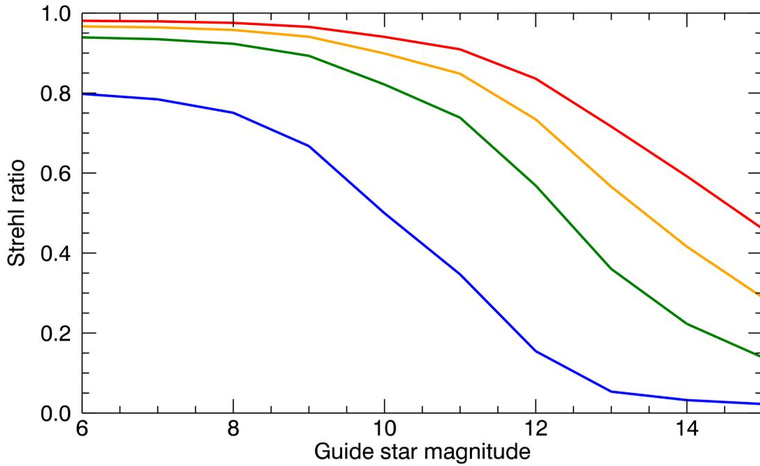
Figure 19: Strehl versus guide star R-magnitude for a closed-loop 7x7 actuator DM system with an  $r_0$  at 550 nm of 0.20 m. The four colors represent R (blue), J (green), H (orange) and K (red).
