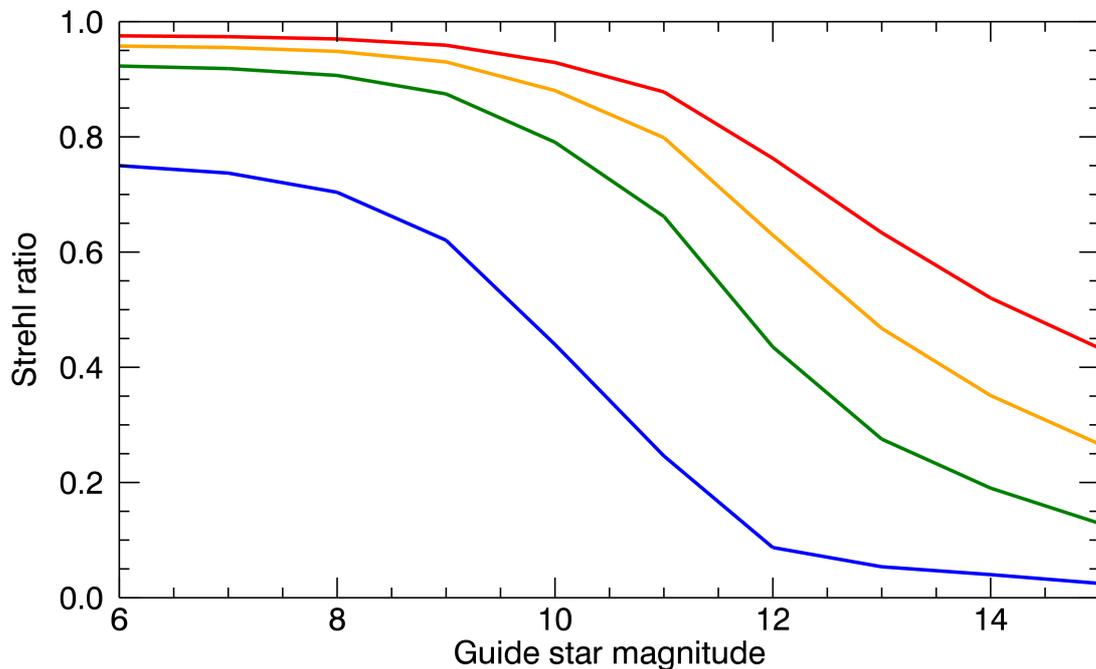
Figure 16: Strehl versus guide star R-magnitude for a closed-loop, 7x7 actuator DM system with an  $r_0$  at 550 nm of 0.20 m. The four colors represent R (blue), J (green), H (orange) and K (red).
