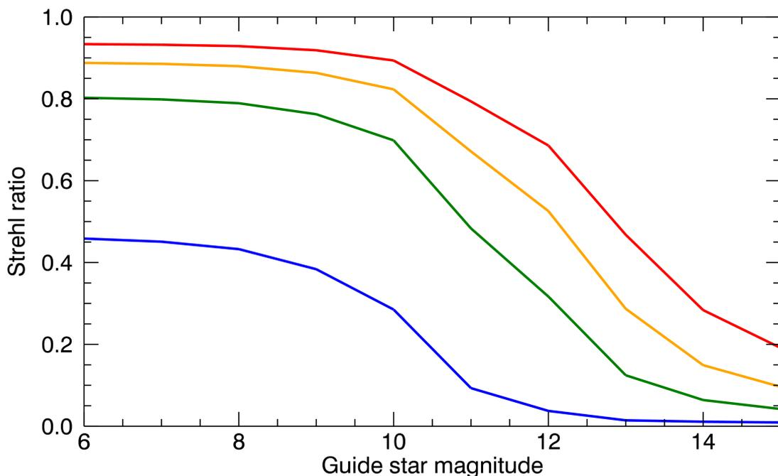
Figure 18: Strehl versus guide star R-magnitude for a closed-loop 7x7 actuator DM system with an  $r_0$  at 550 nm of 0.10 m. The four colors represent R (blue), J (green), H (orange) and K (red).
