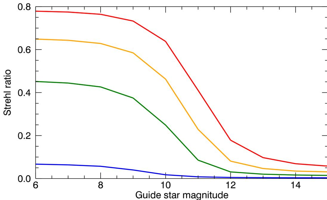
Figure 14: Strehl versus guide star R-magnitude for a closed-loop 7x7 actuator DM system with an  $r_0$  at 550 nm of 0.05 m. The four colors represent R (blue), J (green), H (orange) and K (red).
