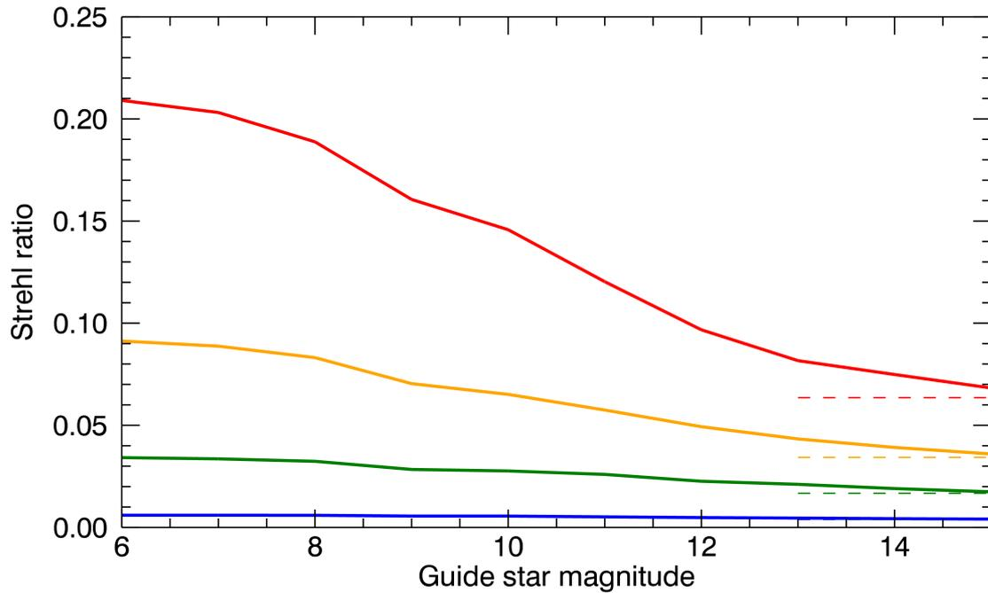
Figure 5: Strehl versus guide star R-magnitude for an open-loop tip-tilt system with an  $r_0$  at 550 nm of 0.05 m. The four colors represent R (blue), J (green), H (orange) and K (red) and the dashed lines show the performance with no correction.
