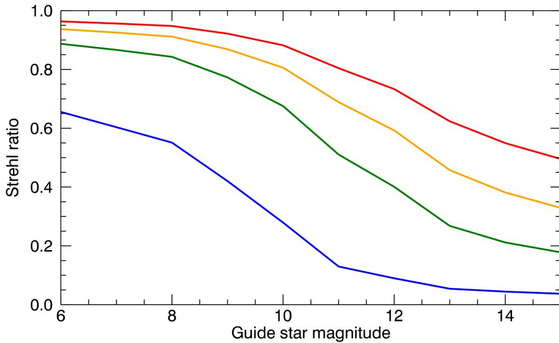
Figure 13: Strehl versus guide star R-magnitude for an open-loop 7x7 actuator DM system with an  $r_0$  at 550 nm of 0.20 m. The four colors represent R (blue), J (green), H (orange) and K (red).
