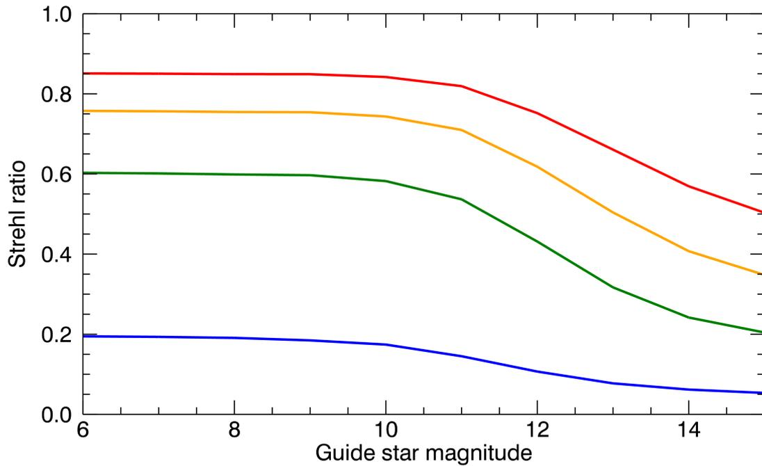
Figure 10: Strehl versus guide star R-magnitude for a closed-loop tip-tilt system with an  $r_0$  at 550 nm of 0.20 m. The four colors represent R (blue), J (green), H (orange) and K (red).
