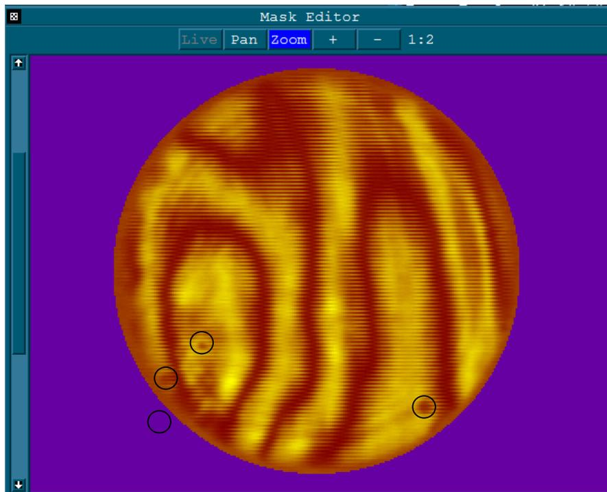
Figure 3. Area of data acquired for one particular part, showing locations of very small pits present on the 12" TF, enlarged due to the defocusing effect of the very long cavity. One circle is not in the measured area of this particular piece, but is in the measured area of others.
