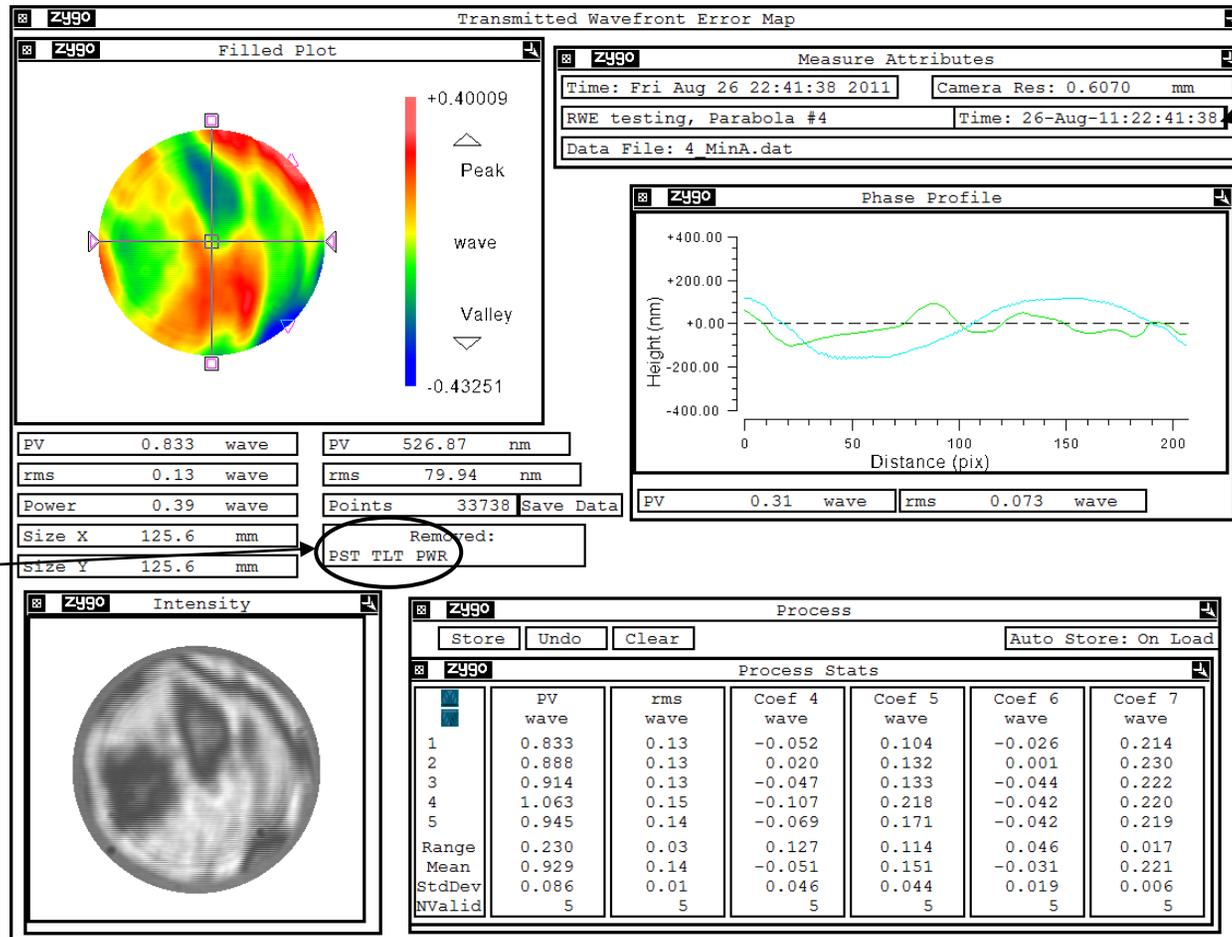
Filled Plot: This shows the shape of the wavefront after it has traveled through your test part. High (red) areas indicate higher areas of the test part.
