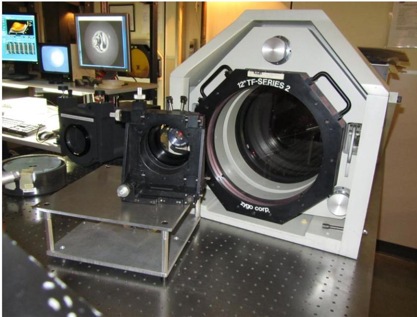
*Figure 2. Photos of setup used. Photo at left, taken from parabola position, shows 12" TF with returning RS mounted just behind parabola focus. Lower photo shows parabola mounted with 1/2" wide polished ring mounted to it. Parabola was adjusted with ring perpendicular to outgoing beam before fine-tuning was performed to minimize aberrations.*
