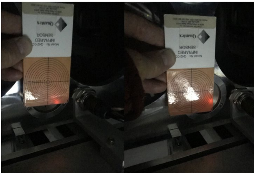
Figure 5: Showing how to check the beam using the edge of the card. One important step is now shown very well. Once the center of beam is set to the edge of the card, you need to look to see if the edge then lines up to the center of the hole.
