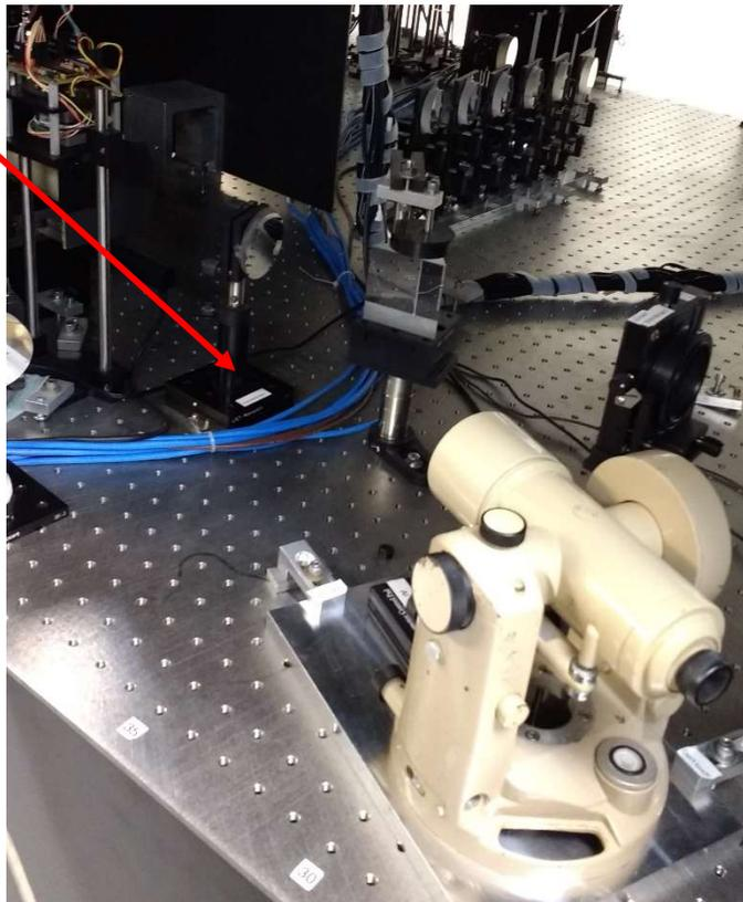
CHANCAM can see the two beams - selected with “VIS-beams” beam sampler stage - reflected back by the BIG-retros.
