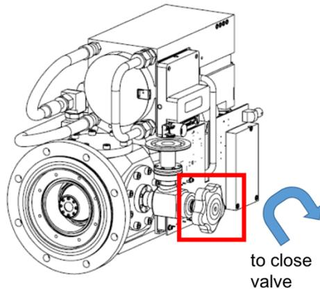
Fig 2: Camera schematic showing location of camera valve and direction of rotation one must use to **close** valve. To open the valve, rotate the knob so that the top moves towards the front of the camera and the bottom moves away.
