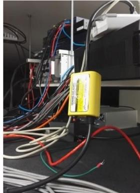
Controller of the **ion pump**, showing the blue power button and the High Voltage red button:
