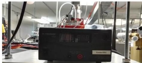
Pfeiffer Vacuum turbo pump (hereafter called the **turbo pump**) in red, together with the electromagnetic valve in black:
