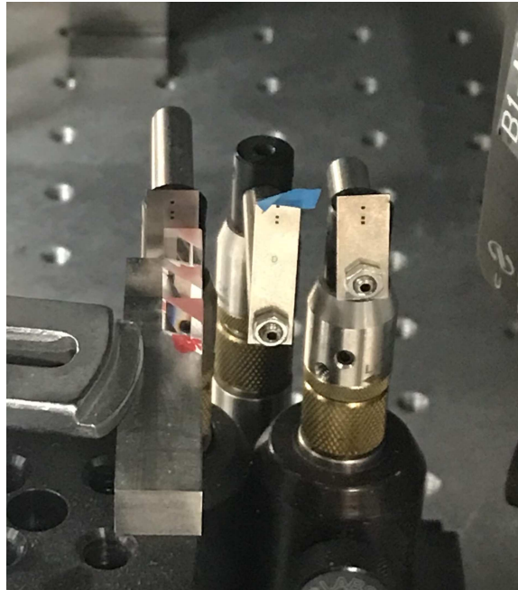
Figure 5.8: This image shows the three right-angle prisms that direct the PAVO beams into the mask holes drilled into a metal sheet. The left-most mask stage is used for PAVO observations. When the mask is "IN," the starlight from each telescope will pass through one of these mask holes (Beam 1 on bottom, Beam 2 in middle, Beam 3 on top; note that this order is reversed from where they appear on the detector).
