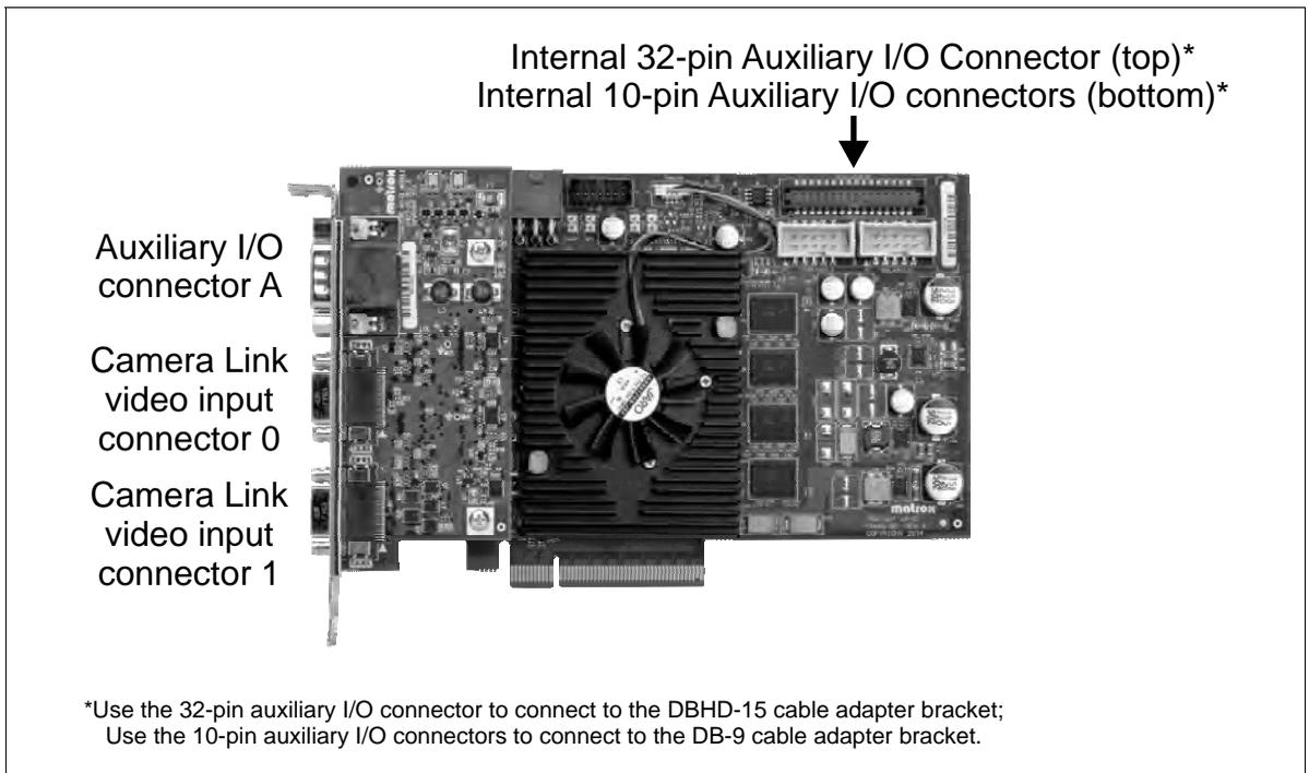
On the Matrox Radient eV-CL cable adapter brackets, there are either two DBHD-15 auxiliary I/O connectors or one DB-9 auxiliary I/O connector; these allow you to access the signals of the internal auxiliary I/O connector from outside the computer enclosure.
