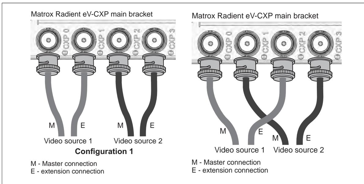
Matrox Radiant eV-CXP communicates with the video sources to identify which video source is connected to which input connectors.
