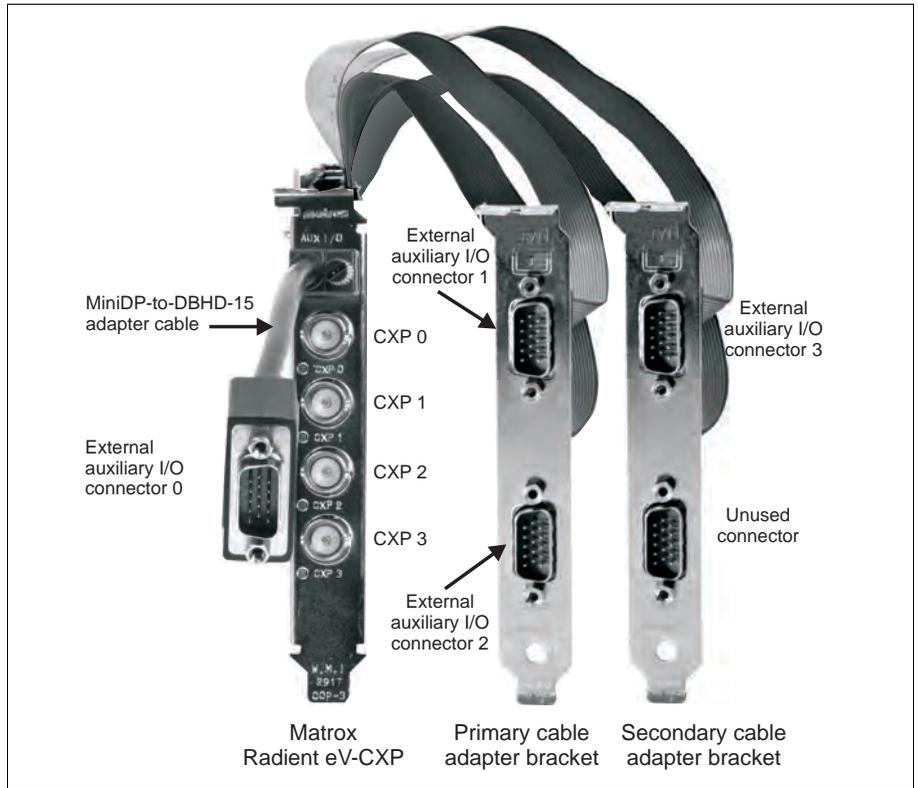
Note that the primary cable adapter bracket is the bracket that you attach to internal auxiliary I/O connector 1, and the secondary cable adapter bracket is the bracket that you attach to internal auxiliary I/O connector 2.
