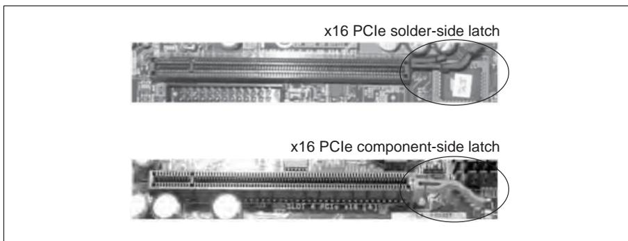
5. Once the input connectors are in the opening of the chassis, press the board firmly but carefully straight down into the connector of the slot.
