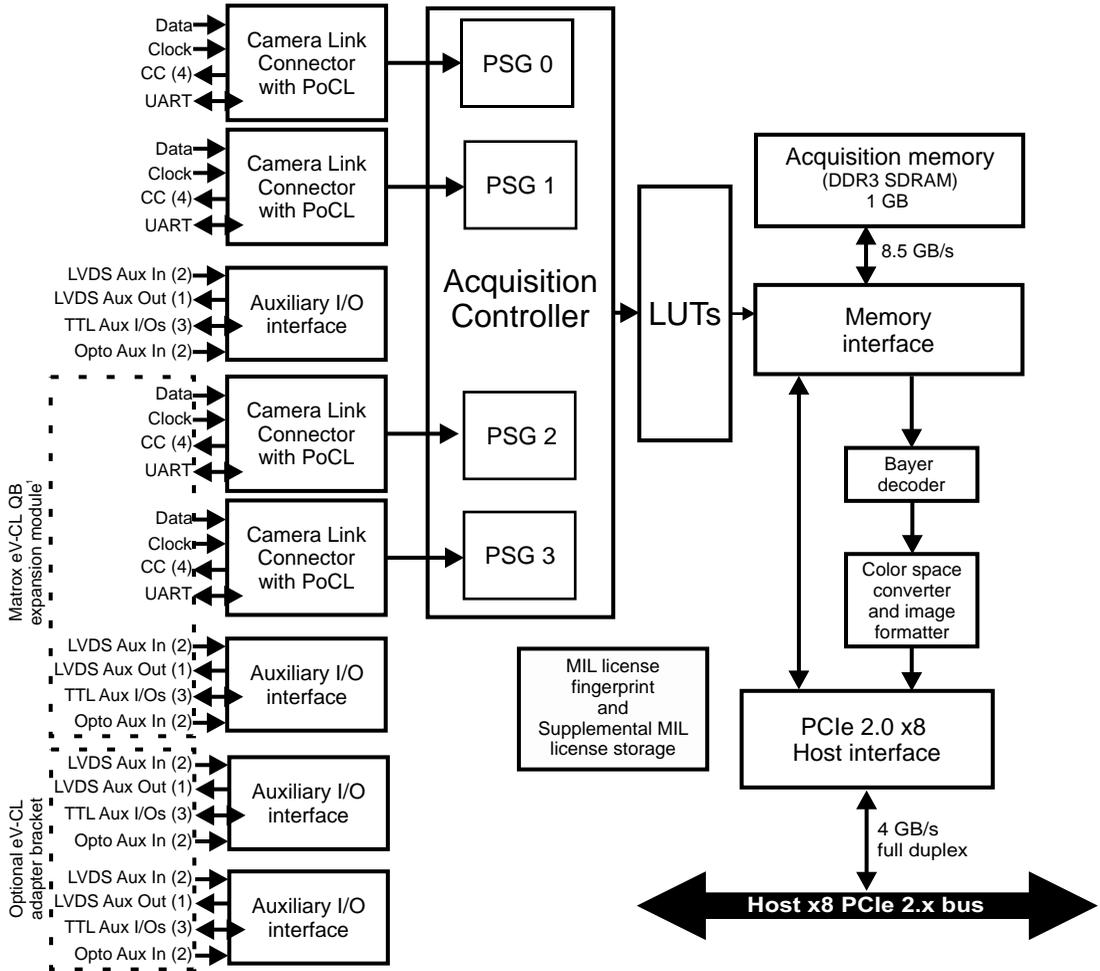
\*Note that, without the expansion module, this is a flow diagram of Matrox Radiant eV-CL DB. With the expansion module, this is a flow diagram of Matrox Radiant eV-CL QB. eV-CL DB is not upgradable to eV-CL QB; the eV-CL DB does not have the required connector for the eV-CL QB module.
