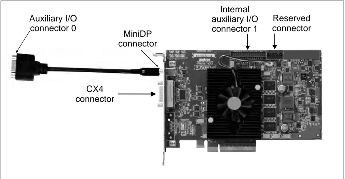
The MiniDP-to-DBHD-15 adapter cable connects to the MiniDP connector on the main bracket. The DBHD-15 connector at the end of this cable is called external auxiliary I/O connector 0.
