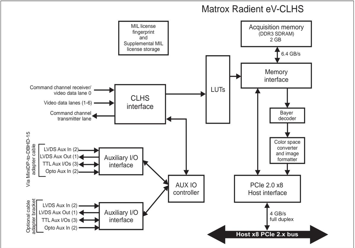
Matrox Radiant eV-CLHS supports a single CLHS link to a video source that transmits data at 3.125 Gbits/sec per video data lane between the video source and frame grabber. A CLHS link contains all the connections and components to capture from one video source.
