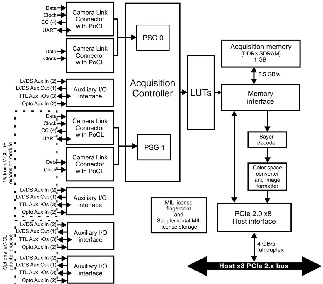
\*Note that, without the expansion module, this is a flow diagram of Matrox Radiant eV-CL SF. With the expansion module, this is a flow diagram of Matrox Radiant eV-CL DF. eV-CL SF is not upgradable to eV-CL DF; the eV-CL SF does not have the required connector for the eV-CL DF module.
