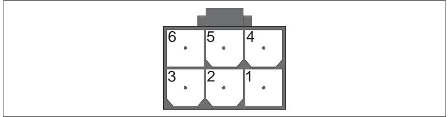
The pinout for the PCIe auxiliary power connector is as follows:
