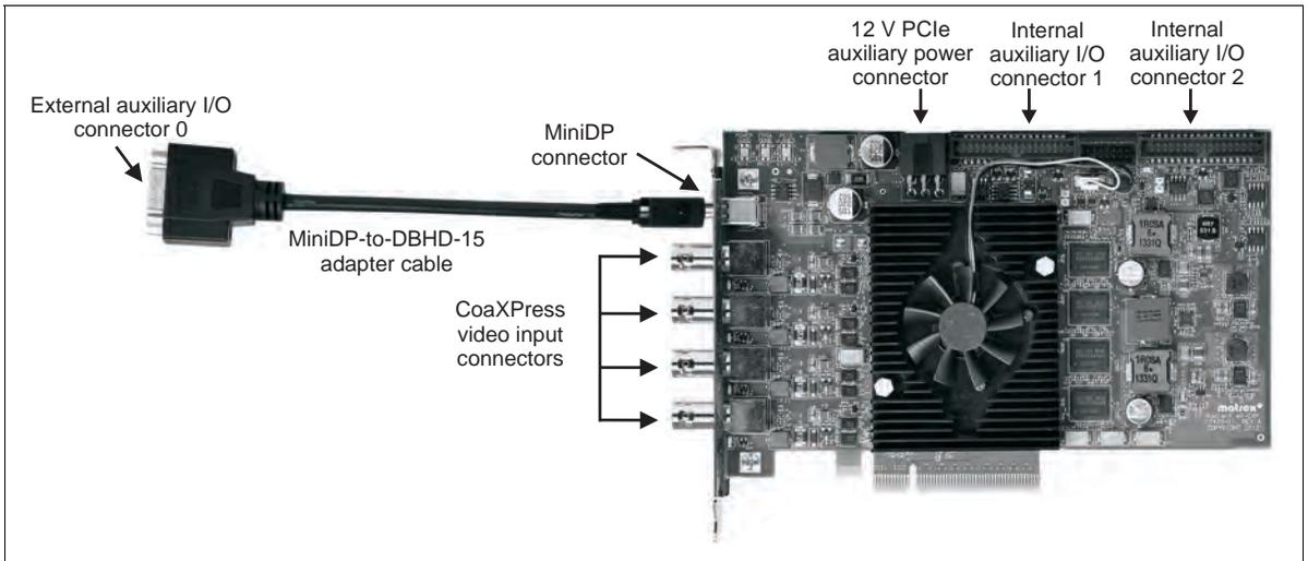
The MiniDP-to-DBHD-15 adapter cable connects to the MiniDP connector on the main bracket. The DBHD-15 connector at the end of this cable is called external auxiliary I/O connector 0.
