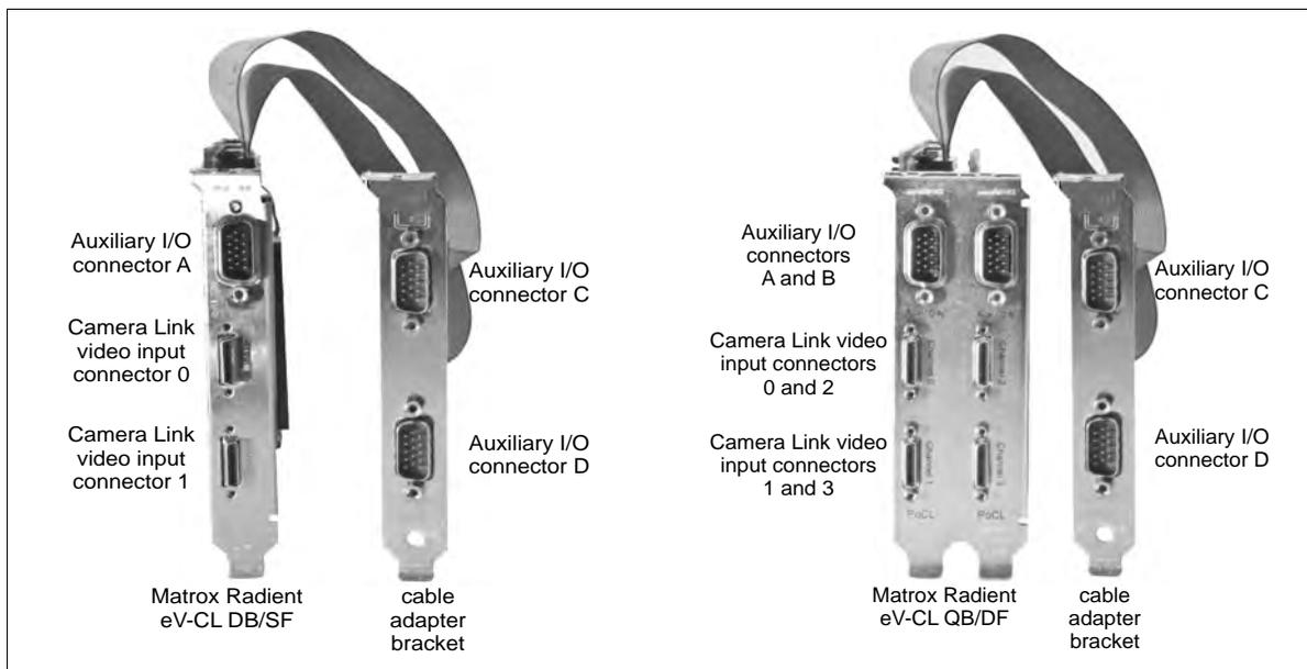
Attach video sources to Matrox Radiant eV-CL as follows:
