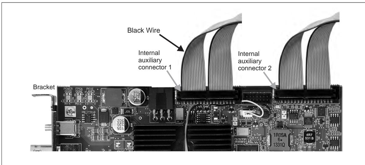
3. Slide the bracket of the cable adapter bracket into the opening at the back of the selected slot.
