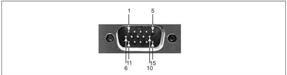
The pinout for auxiliary I/O connector 0 is as follows. Auxiliary I/O connector 1 has the same pinout as auxiliary I/O connector 0, except you must add 8 to the number at the end of their hardware signal name and MIL constant. For example, AUX(TRIG)\_TTL\_IO\_4 on auxiliary I/O connector 0 is AUX(TRIG)\_TTL\_IO\_12 on auxiliary I/O connector 1.
