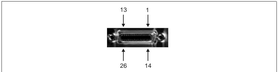
The number of Camera Link video input connectors and their pinout depends on the version of Matrox Radient eV-CL and the configuration. The pinout of these connectors follows the Camera Link standard.
