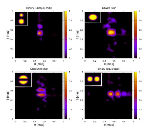
Figure 1. Four examples of images reconstructed from SII data as would be recorded with an array that operates at a wavelength of  $\sim 400\,\mathrm{nm}$  with one hundred telescopes and a telescope separation of  $\sim 100\,\mathrm{m}$ . The pristine image is shown at the top left in each example. The images were produced [8] using an algorithm based on the Cauchy-Riemann equations [9]. The analysis does not yet include a realistic noise component, which is still actively being investigated.
