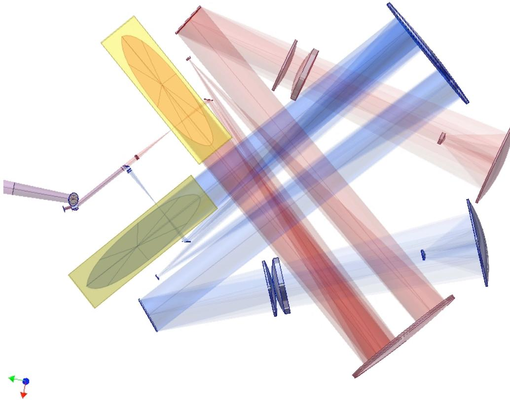
**Figure 4- Top view of MTHR’s high-resolution mode.**
