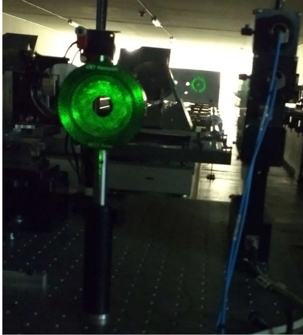
Figure 5. The placement of the additional iris for guide rail alignment.
