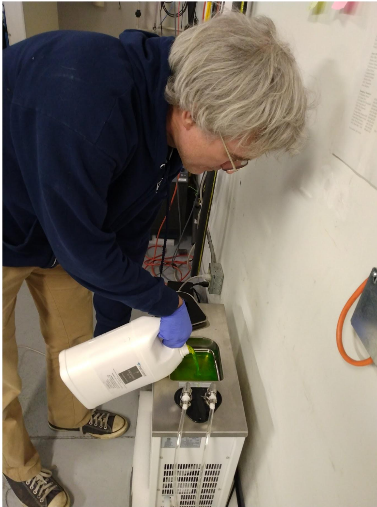
Figure 8 Water chiller is used to cool down the camera. The photo was taken while Prof. John Monnier filled the water chiller with 50% mix of water and glycol.
